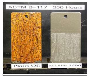
This ASTM B-117 salt spray test shows that a coating of Eco-Line® 3690 protects metals for 300 hours in 100% humidity with no rust. Further tests have shown the same results with over 2,000 hours logged.
